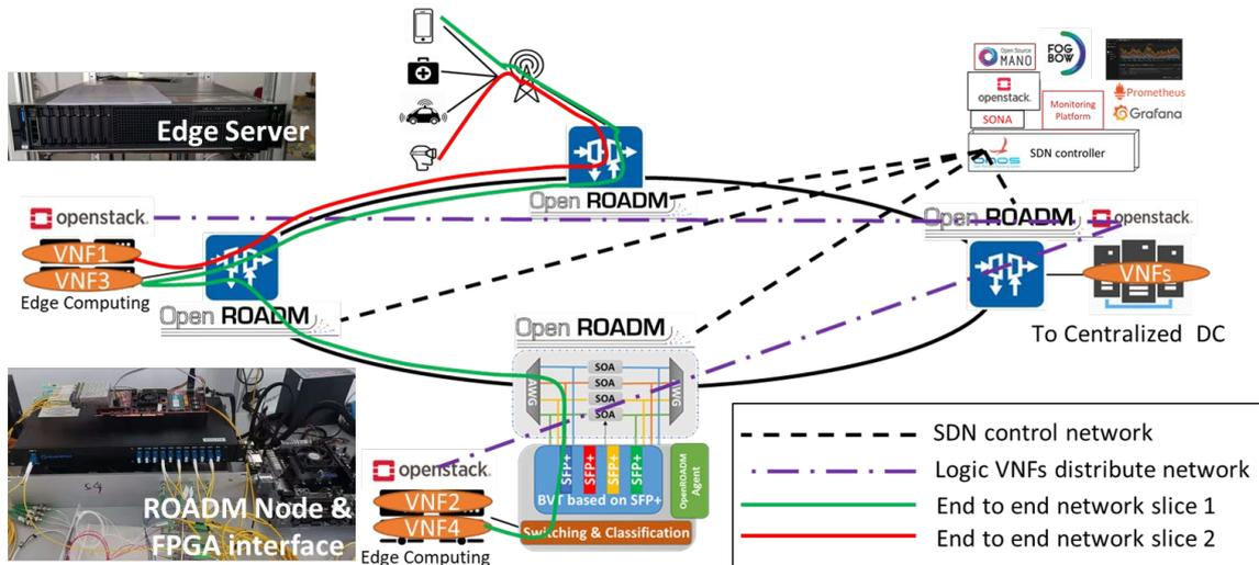
Fig. 1. Disaggregated and sliceable optical metro access network
