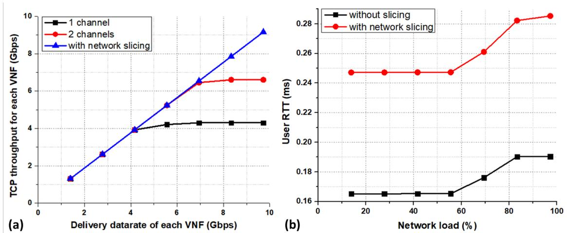
Fig.2 (a) TCP throughput of each VNF versus the delivery datarate (b) User experienced RTT in different network operation case
