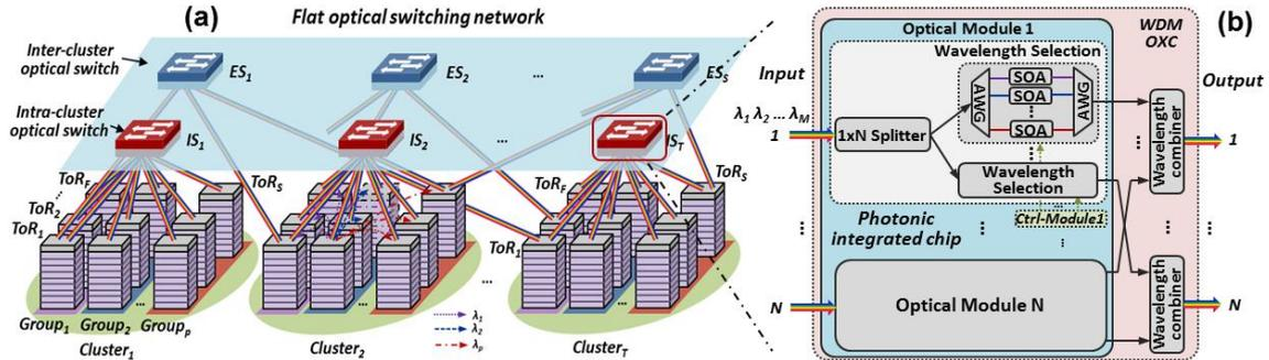
Fig. 1: (a) Schematic of a flat DCN topology. (b) Schematic of the WDM optical cross-connect. TOR: Top Of the Rack (switch), refers to the servers organized in racks and cluster of racks.
