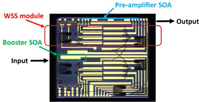
Fig. 2: Microscope image of the modular WDM photonic switch.
