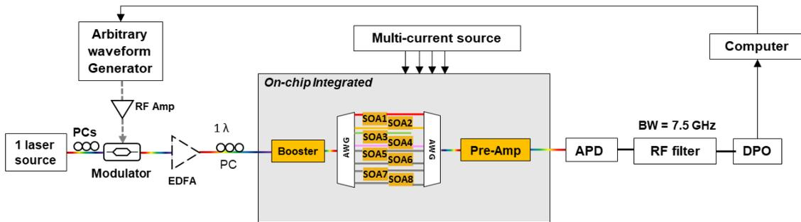
Fig. 3: Experimental set-up employed to assess the performance of the WDM photonic switch for DMT modulation format. EDFA: Erbium Doped Fiber Amplifier, APD: Avalanche Photo Diode, DPO: Digital Phosphor Oscilloscope.
