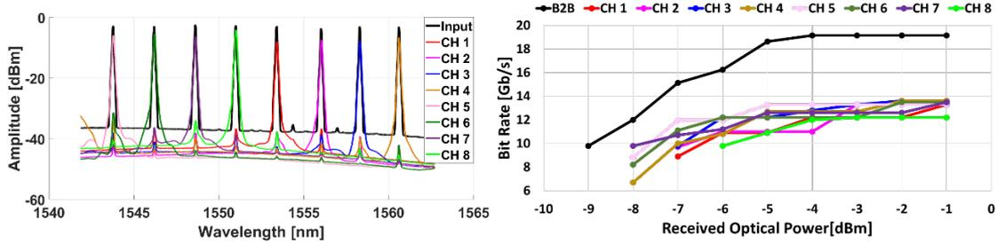
Fig. 4: Optical spectra of the WDM channels switched by the WSS (left). Highest bit rate achievable as a function of received optical power for each channel for DMT modulated traffic (right).
