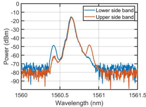
Figure 3: Optical spectrum after the optical single-sideband generator.
