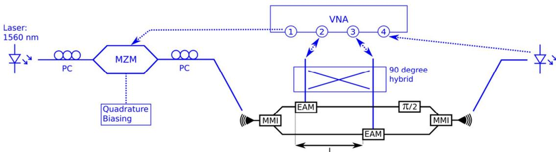
Figure 5: Full duplex measurement setup. (PC: polarization controller; MZM: Mach Zehnder modulator; VNA: vector network analyzer; MMI: multi-mode interferometer.)
