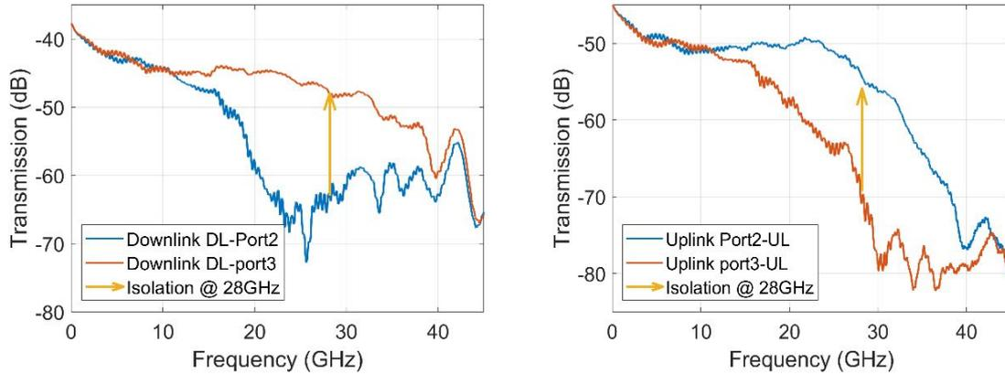
Figure 6: Transmission between the optical downlink/uplink to the respective electrical port and to the isolated port. The isolations at 28GHz are indicated with the arrows.
