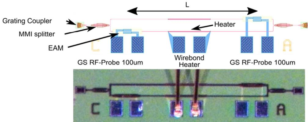
Figure 1: Layout and implementation of the quadrature EAM structure. (MMI: multi-mode interferometer; GS: ground signal.)
