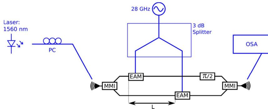
Figure 2: Setup optical single-sideband generation with the quadrature EAM structure (PC: polarization controller; OSA: optical spectrum analyzer; MMI: multi-mode interferometer.)
