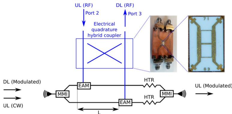
Figure 4: Quadrature modulator. (DL: downlink; UL: uplink; CW: continuous wave; HTR: heater; MMI: multi-mode interferometer..)
