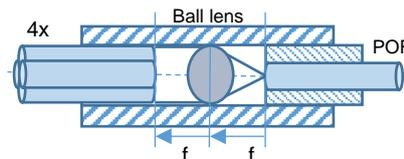
Fig. 3. Principle of operation from the MUX developed.
