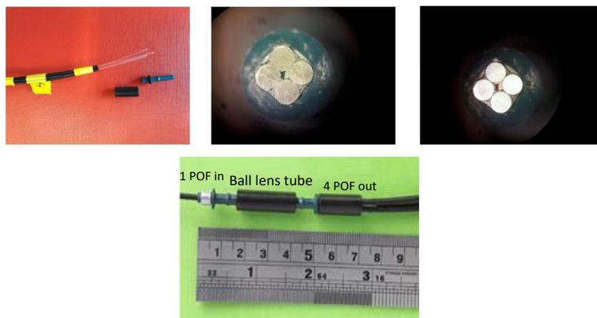
Fig. 4. MUX prototype.
