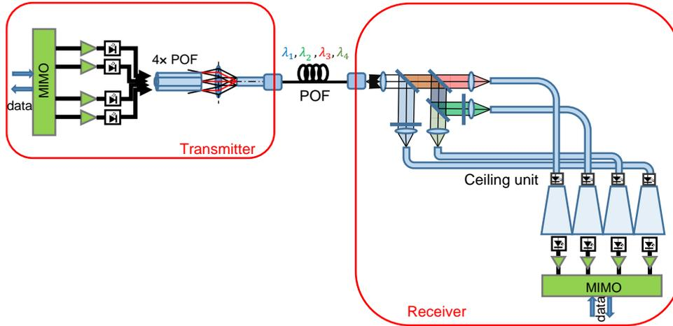
Fig. 2. Principle of operation of the WDM-POF.
