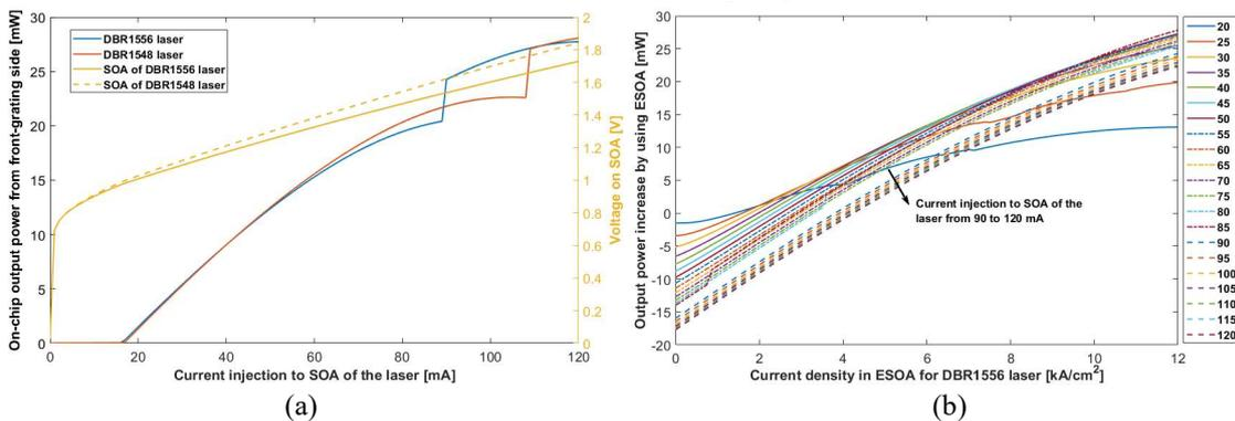
Figure 4. (a) LIV-curves of two DBR lasers measured separately from the device. (b) Each curve shows with a specific output power from DBR1556 nm laser, the power increase by using ESOA with different current density. The legends show the current injection to the SOA of the laser, and the relevant laser output power could be found from (a).
