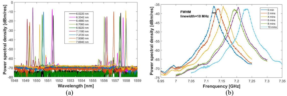
Figure 2. (a) Optical spectra of THz beat notes measured from the top device in Figure 1. The wavelength separation of these two laser peaks is from 6.02 to 7.69 nm. (b) Microwave signal at frequency of 7.13 GHz by using on-chip RF photodiode measured from the bottom device in Figure 1.
