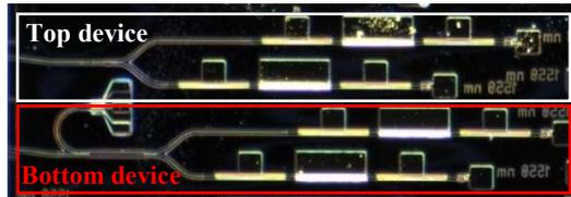
Figure 1. Microscope picture of two devices from the first PIC. Top device: Two-combined DBR laser with Bragg wavelengths of 1550 and 1558 nm respectively, Bottom device: Two-combined DBR laser with the same Bragg wavelength of 1550 nm, and one of the output ports connecting with a RF photodiode.
