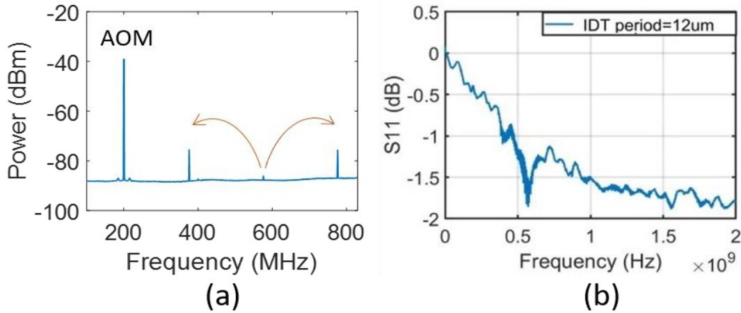
**Figure 5:** (a) The two sidebands appear from the mixing. The maximum sideband amplitude (phase modulation) occurs at RF frequency of 576 MHz (b) The  $S_{11}$  parameter from the same IDT shows dip at 576 MHz. These results prove the excitation of SAW on the PZT and the first order mode frequency of SAW is 576 MHz for the given IDT structure.
