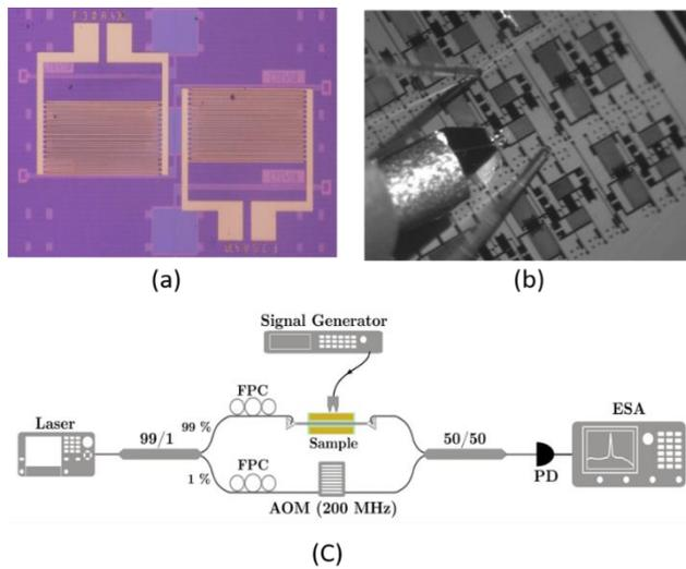
**Figure 4:** (a) A microscopic image of a silicon TE waveguide (width 550nm) integrated with an IDT (period 12  $\mu\text{m}$ , 20 periods, aperture size 180 $\mu\text{m}$ ). (b) camera view shows the landing of a GS probe (100 $\mu\text{m}$  pitch) on IDT electrode pads. Two optical fibers are aligned with the grating couplers for the optical transmission measurement. (c) A heterodyne-setup is used for the measurement of the phase modulation in a single waveguide.
