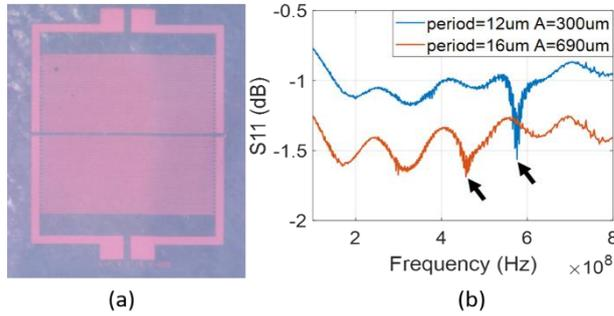
**Figure 3:** (a) Microscopic image of an IDT- IDT system. We apply poling voltage on the IDT for 30-40 min and then measure the reflection  $S_{11}$  with VNA. (b)  $S_{11}$  shows that now for the IDT period 12  $\mu\text{m}$ , the SAW frequency has almost doubled (310MHz to 590 MHz) and it varies consistently with the IDT period change. The ripples in the  $S_{11}$  signal is due to the cavity effect from RF
