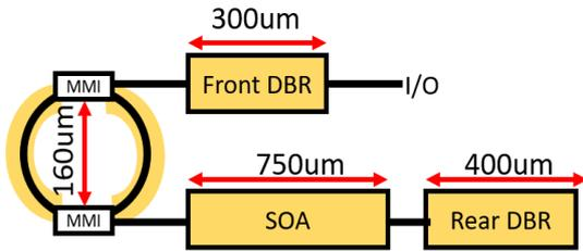
Figure 1: Dual DBR laser with intra ring resonator. Gold representing tuneable
