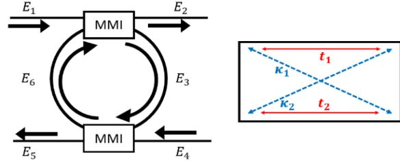
Figure 2: a) MMI coupler ring resonator, b) MMI coupler indicating cross and bar states.
