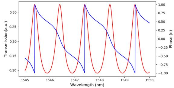
Figure 4: Transmission and phase of the electric field transmitted through ring resonator using 50:50 MMI coupler.
