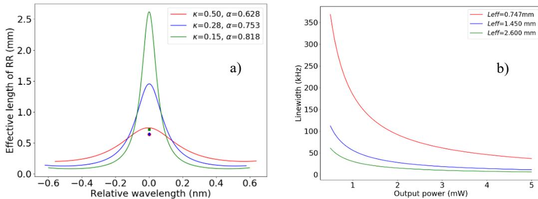
Figure 5: a) Effective length of Ring resonator against the normalised wavelength, b) Intrinsic linewidth against output power for the DBR RR laser with different effective lengths.
