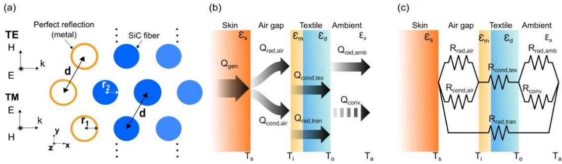
Figure 2 – (a) Electromagnetic modeling. The polarisation convention and incidence direction are indicated. The pattern is repeated in the vertical  $y$ -direction. (b) Main heat flow channels when the fabric covers skin, with an air gap in between (shown in cooling mode). (c) Thermal circuit model.  $T_{s/a/i/o}$  are the temperatures of the skin, ambient, inner and outer textile layers, and  $\epsilon_{s/a/i/o}$  are their emissivities.
