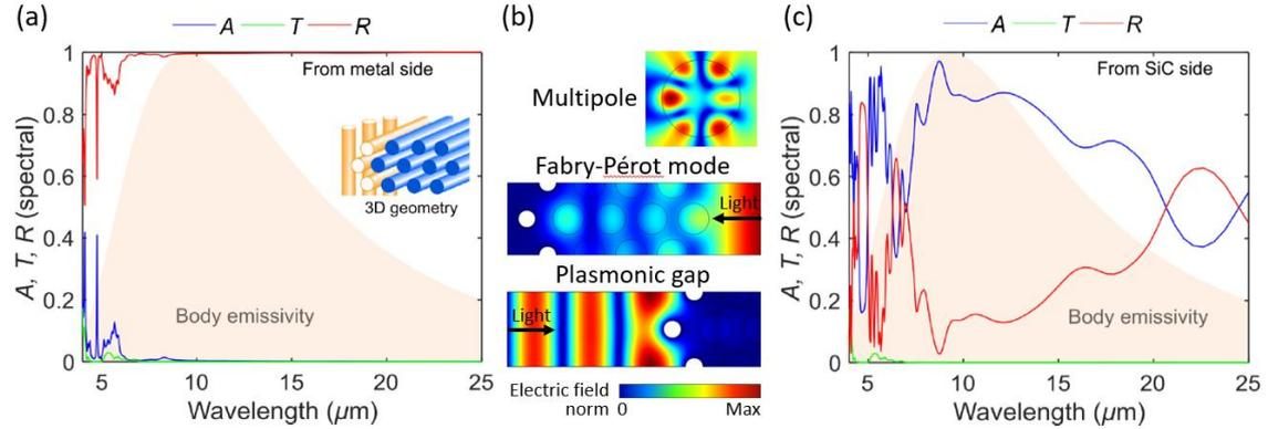
Figure 3 - Unpolarized absorptivity, transmissivity and reflectivity of the best (3D) Janus-yarn structure ( $r_1 = 0.6\mu\text{m}$ ,  $r_2 = 1.125\mu\text{m}$ ,  $d = 3\mu\text{m}$ , 3 layers of SiC fibers), from the metallic (a) and dielectric (c) sides. (b) Field profile examples of the plasmonic gap, a Fabry-Pérot mode and a multipole resonance.
