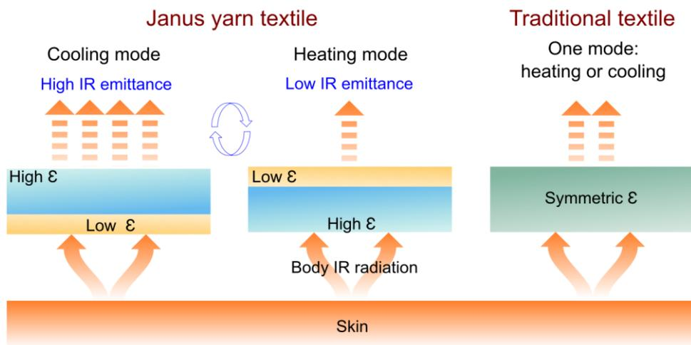
Figure 1 - Janus yarn textile working principle. When a high emissivity layer faces the ambient, the fabric is in cooling mode (left). Once the textile is flipped and the low emissivity layer faces outside, the fabric is in heating mode (center). In contrast, a traditional textile (right) only has one mode: heating or cooling.
