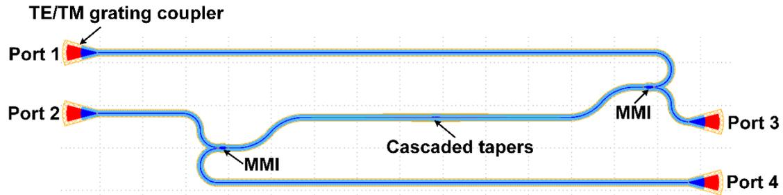
Fig. 5. Schematic of the four-port measurement structure
