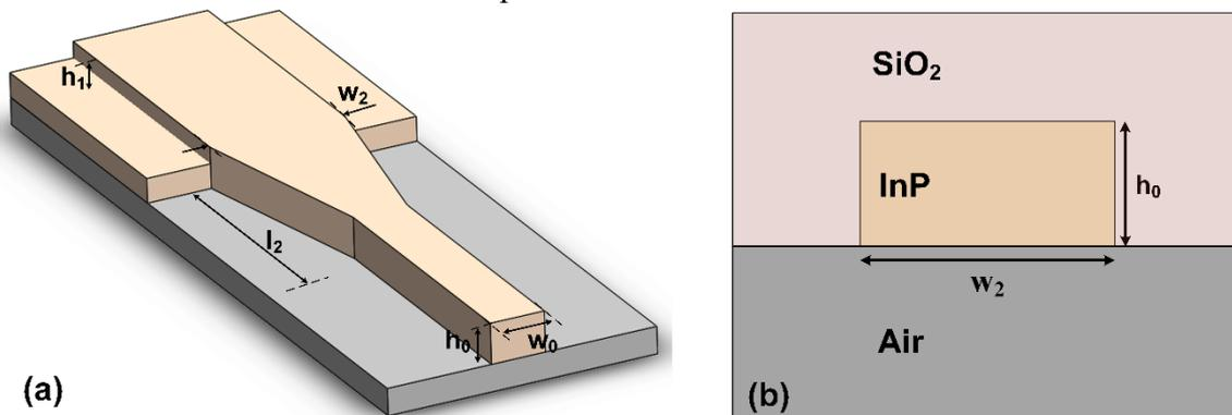
Fig. 2 The butt-jointed taper (a) the schematic (b) the cross-section in the taper section
