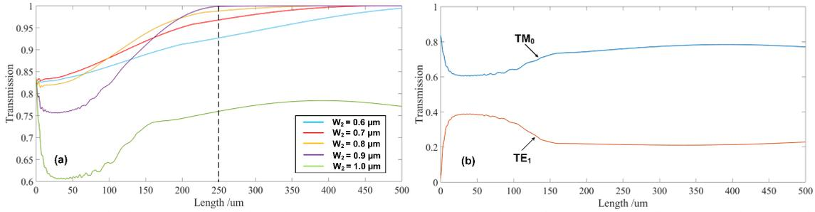
Fig. 3 Simulation results of the bi-level taper (a) transmission of  $\text{TM}_0$  mode (b) transmission of  $\text{TM}_0$  mode and  $\text{TE}_1$  mode when  $w_1$  is  $1.0 \mu\text{m}$
