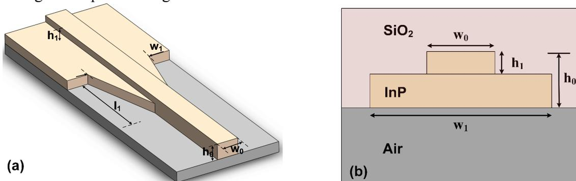
Fig. 1 The bi-level taper (a) the schematic (b) the cross-section in the taper section
