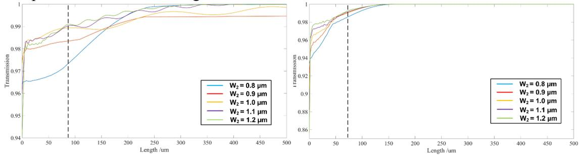
Fig. 4 Simulation results of the butt-jointed taper (a) transmission of  $\text{TM}_0$  mode (b) transmission of  $\text{TE}_0$  mode
