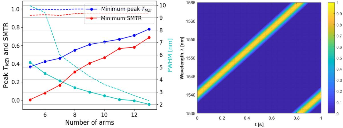
Figure 3: (a) Minimum peak transmission, SMTR and FWHM in solid and maximum corresponding values in dashed lines, with increasing number of arms. (b) Transmission of CWT filter in time tuned for 30 nm.
