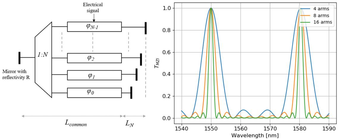
Figure 1: (a) The schematic of CWT filter for  $N$  arms configuration. (b) Transmission of CWT filter resulting in a wavelength dependent sinc function, for varying arm numbers.
