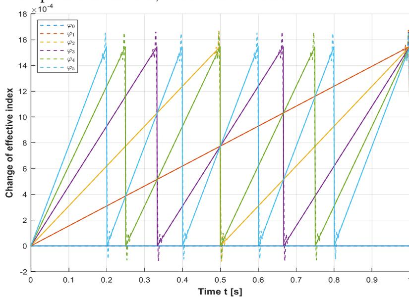
Figure 2: The sawtooth signals ideal in dashed and bandwidth limited in solid lines. The overlap of simultaneous resets of  $\varphi_4$  and  $\varphi_2$  can be observed at  $t=0.5$  s.
