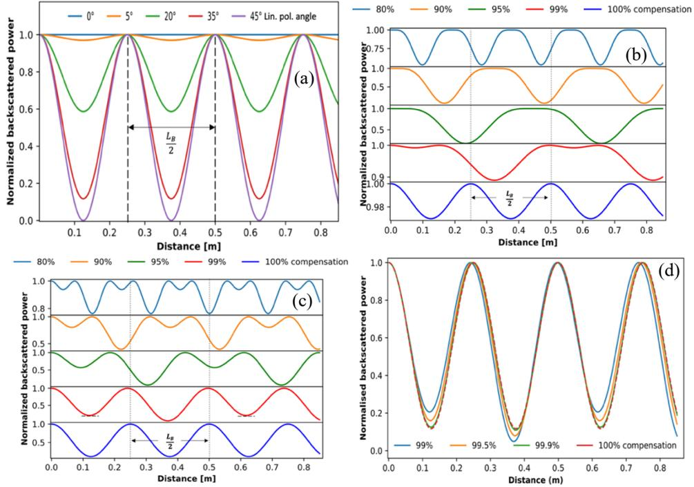
Fig. 2 (a) Effect of linear SOP azimuth, when spinning effect is completely cancelled.
