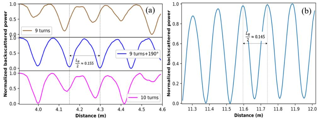
Fig. 3: POFDR trace based  $L_B$  measurement of (a) spun fibre and (b) unspun fibre drawn from the same preform
