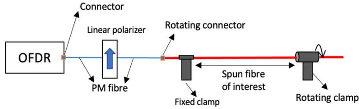
Fig.1. POFDR setup for  $L_B$  measurement of spun fibre
