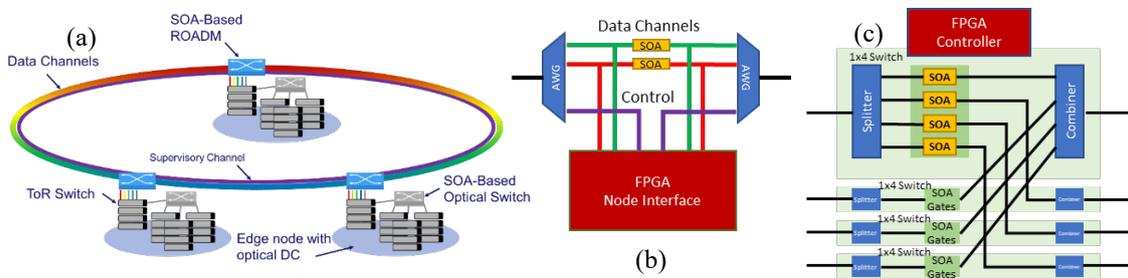
Fig 2. – (a) Proposed optical ring network interconnecting edge data center nodes, (b) SOA-based ROADM and (c) SOA-based intra-datacenter optical switch (for simplicity only one 1x4 instance is shown in detail).
