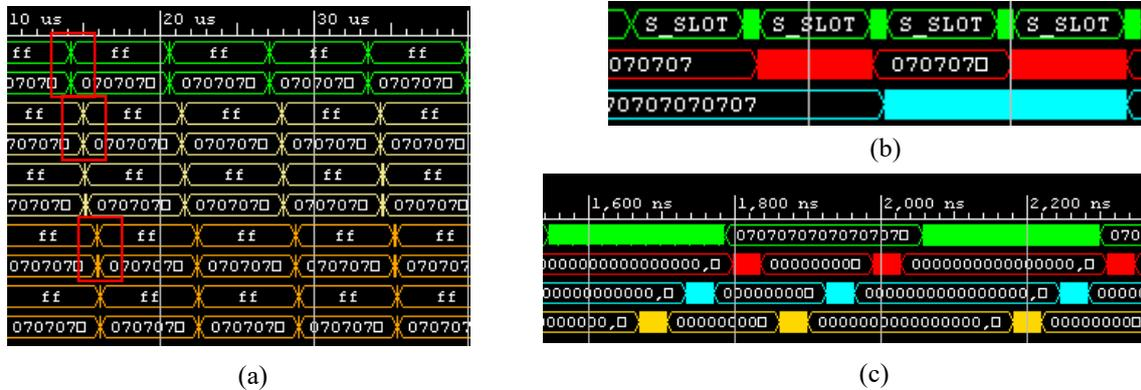
Fig 3. – Data and control simulated FPGA traces in different scenarios in the network: (a) forwarding of control packets, (b) data slots in two channels and (c) distribution by gateway ToR of incoming time-slotted data to different optical ports.
