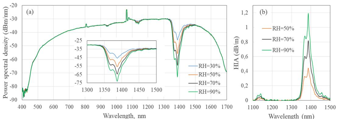
Fig. 2 Transmission spectra of 23-m CYTOP fiber sample at different RH levels (a); HIA calculated relatively 30 % RH level (b).
