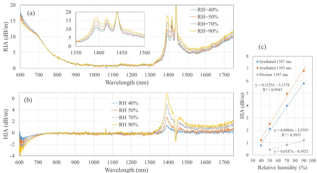
Fig. 3 Radiation induced attenuation of CYTOP fiber received 17.5 kGy dose of gamma radiation for different levels of relative humidity (a); humidity induced attenuation (b); Peak HIA versus relative humidity for pristine and irradiated POF (c).
