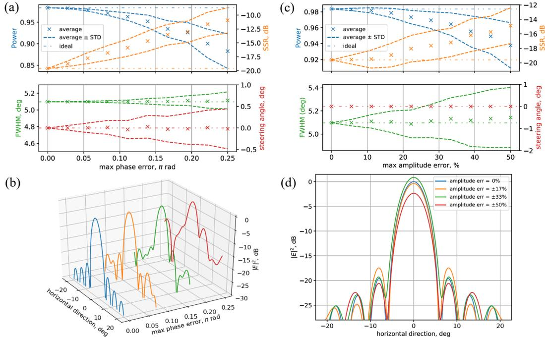
Figure 2: (a) Ratio of power in the main beam, SSR, angular resolution and steering angle at different phase error conditions. (b) Far field profiles with increasing phase error. (c, d) Simulation results for amplitude fluctuations.
