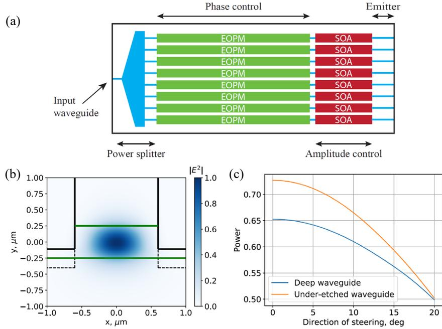
Figure 1: (a) Schematic of the designed OPA. (b) Fundamental TE mode of an under-etched  $1.2\mu\text{m}$ -wide waveguide. The waveguide profile is drawn in black, and its core is highlighted in green; the dashed lines show the profile of an ideal fully etched deep waveguide. (c) Main beam power ratio across  $180^\circ$  steering range for fully-etched and under-etched emitter waveguides.
