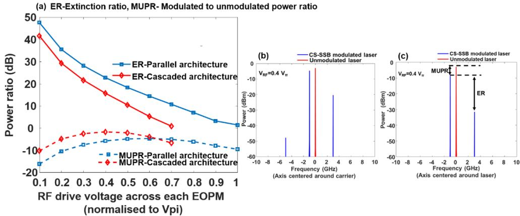
Figure 3 (a) ER (extinction ratio) and MUPR (modulated to unmodulated power ratio) as a function of RF drive voltage in parallel and cascaded MZM architectures. (b) Lower sideband of cascaded architecture at  $V_{RF} = 0.4 V_{\pi}$ , and (c) Lower sideband of parallel architecture at  $V_{RF} = 0.4 V_{\pi}$
