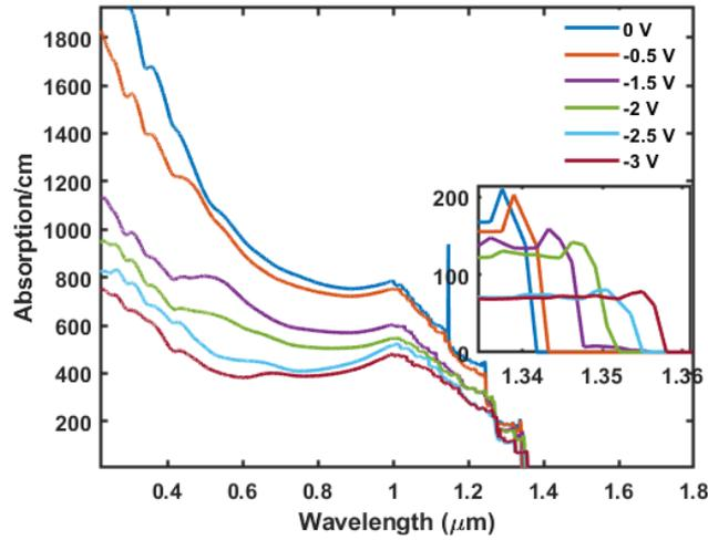
Fig. 3. The absorption curve of the TE mode as a function of wavelength.
