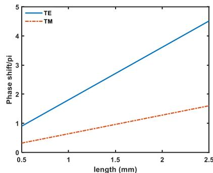
Fig. 5. Phase shift of the TE and TM modes versus the phase shifter length.
