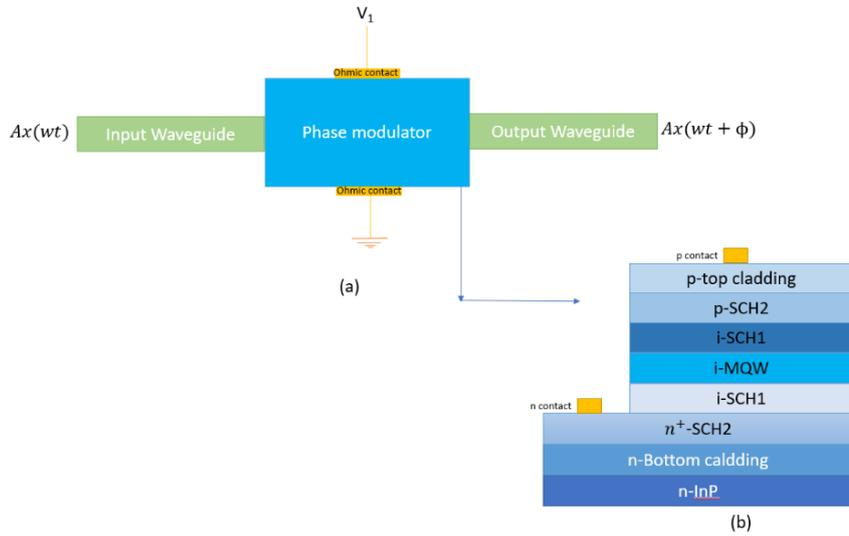
Fig. 1. The phase shifter structure (a) building block and electronic and optical interfaces (b) layer stack.
