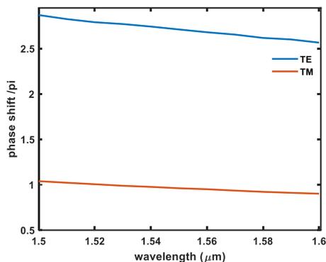
Fig. 4. Phase shift of the TE and TM modes versus wavelength.
