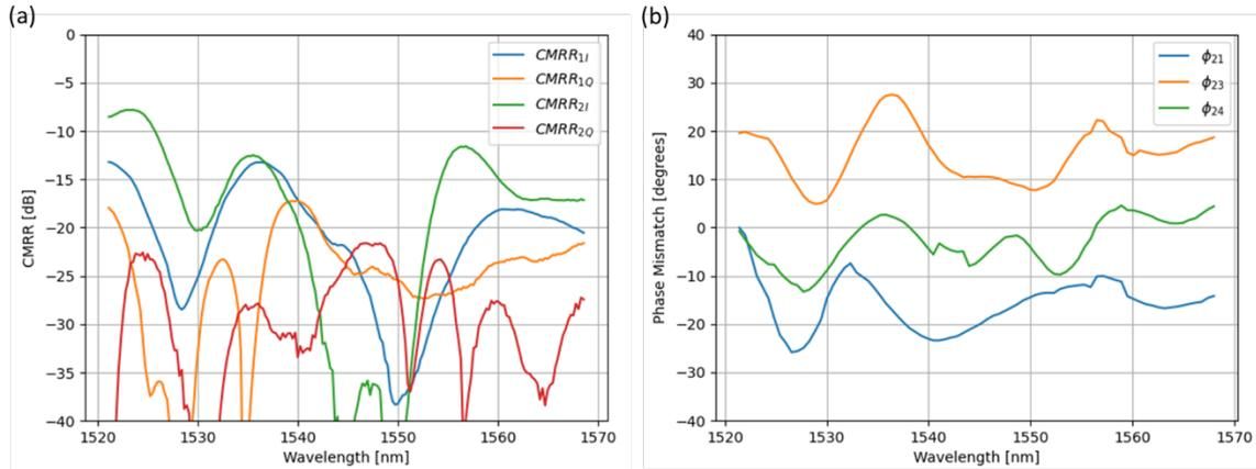
Figure 4 – The calculated (a) CMRR and (b) phase mismatch values
