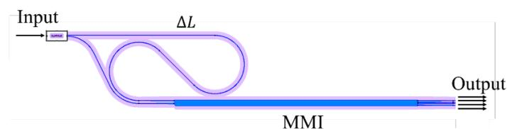
Figure 1 – The layout of the 90° hybrid test structure
