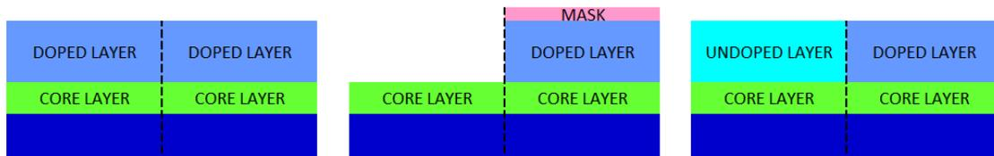
Figure 1 Visualization of the butt-joint process in top waveguide layers
