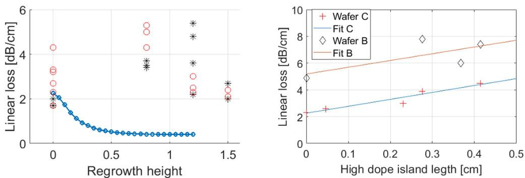
Figure 2: Left side: comparison of real data against simulation. Right: impact of doping on single wafer
