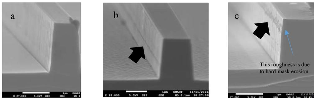
Figure 3 SEM Imaging of waveguide cross section for Wafer D , Wafer C and Wafer B
