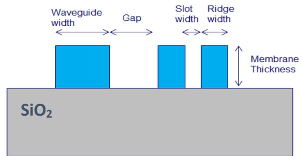
Fig. 2. PBS schematic – Cross section
