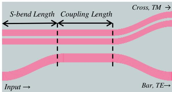
Fig.1. Passive PBS schematic – Top view
