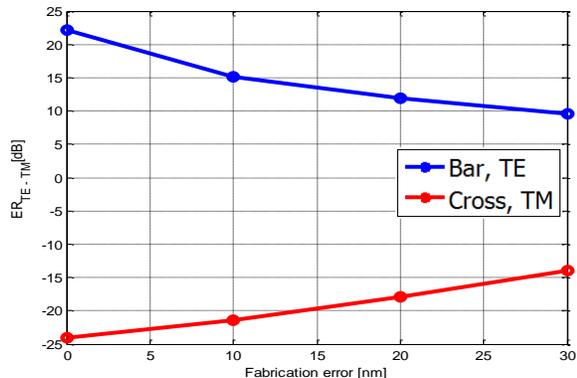
Fig. 4. ER as a function of fabrication error @ 1.55 $\mu$ m.
