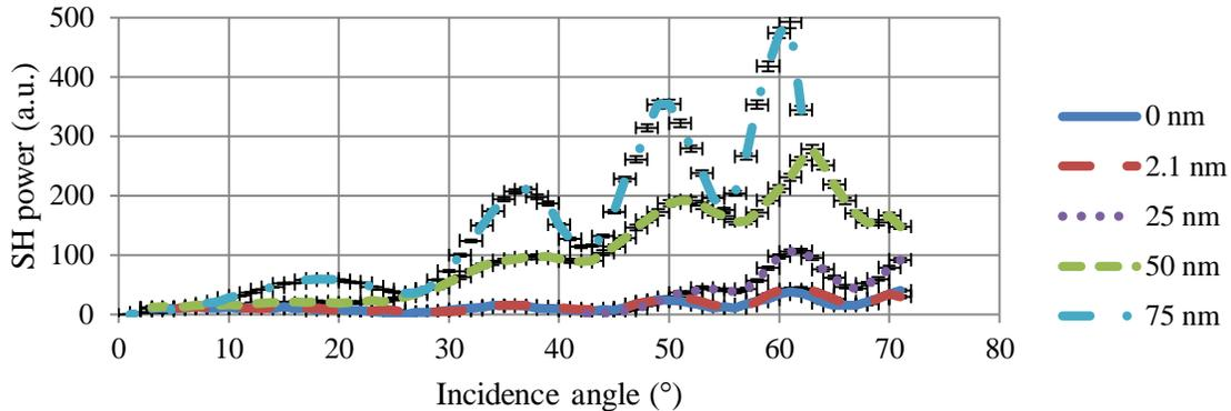
**Fig. 1:** Second-harmonic power measured in function of the incidence angle of the laser beam.  $0^\circ$  corresponds to normal incidence. The results are shown for a blank glass substrate (0 nm), for an ABC stack with a total thickness of 2.1 nm, 25 nm, 50 nm and 75 nm.
