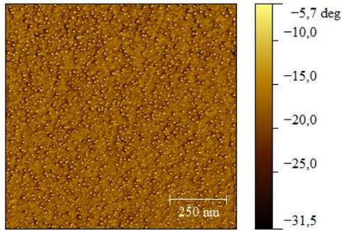
**Fig. 1:** Phase AFM images in intermittent contact mode of a Ag-PVA film doped with 25%  $\text{AgNO}_3$  (w:w). (Thickness: 300 nm). Image size:  $1 \mu\text{m} \times 1 \mu\text{m}$  (256 x 256 pixels).
