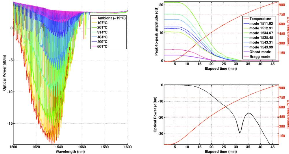
**Fig. 1.** a Transmission spectrum of the TFBG for different temperatures (left), 1.b Evolution of the peak-to-peak amplitude of some resonances measured in transmission (upper right) and 1.c Evolution of the Bragg mode reflected optical power (lower right).
