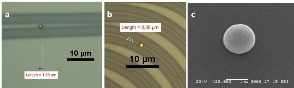
**Fig. 1.** (a) a LIFTed Au droplet on a Si<sub>3</sub>N<sub>4</sub> waveguide (b) a LIFTed Au droplet on a Si<sub>3</sub>N<sub>4</sub> bend waveguide (c) SEM image of on droplet under 45° tilt
