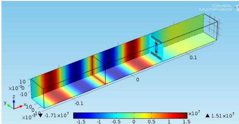
**Fig. 1:** The unit cell of the energy harvesting metamaterial and setup of the numerical simulation
