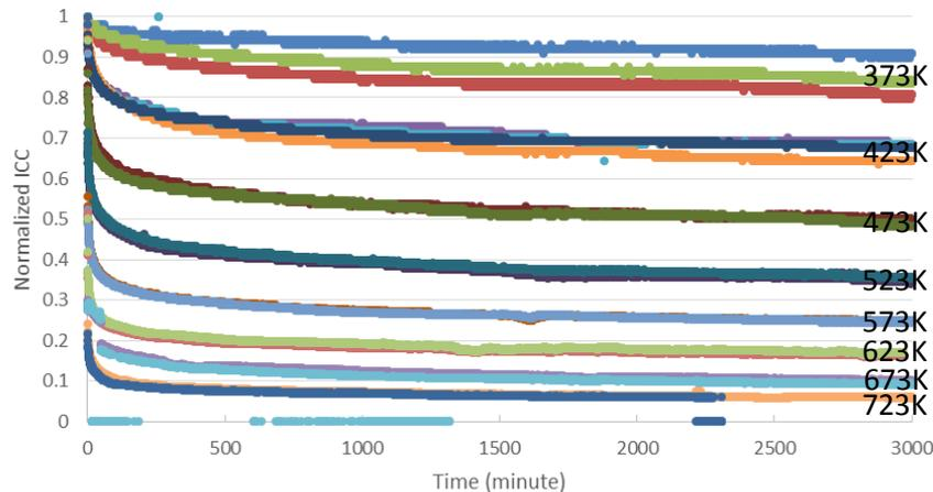
**Fig. 1:** The accelerated aging test results on DTGs.
