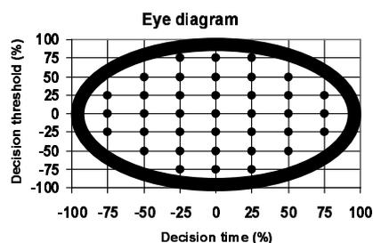
Figure 1: Schematic eye diagram normalized to the bit-rate and to the peak-to-peak signal
