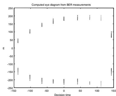
Figure 4: Eye diagram contours from  $10^{-2}$  to  $10^{-16}$  obtained from BER measurements.
