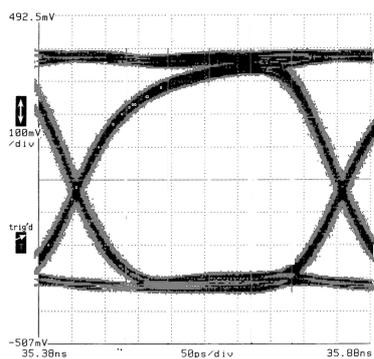
Figure 3: Measured eye diagram on the scope
