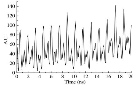
Fig. 7: Pulse train under mode-locking conditions. The 1.3 ns pulse separation equals the cavity roundtrip time.
