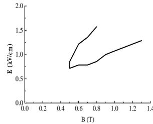
Fig. 3: E-B field region of laser action.
