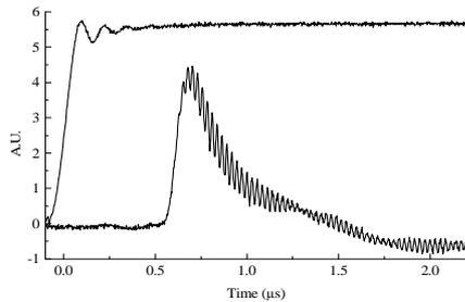
Fig. 6: Time resolved laser output at  $B=0.78$  T observed with a fast Heterostructure detector and the high voltage pulse (upper trace).
