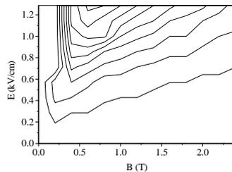
Fig. 2 E-B emission region of small crystal ; each contour line is a 4 mV signal increase from 4 to 36 mv.
