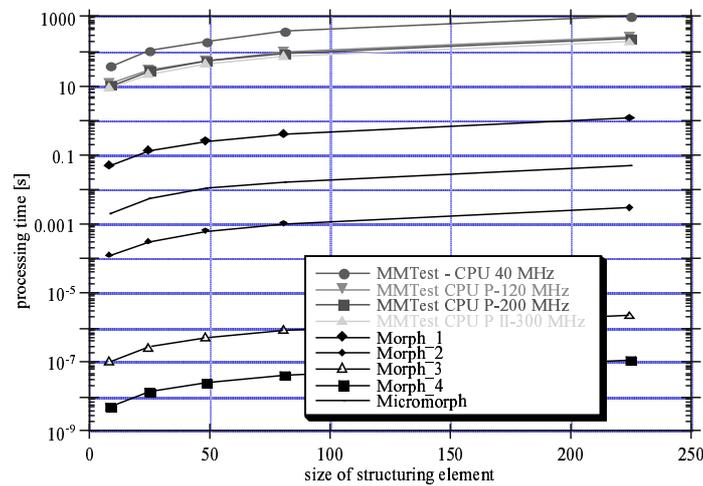
Figure 3 Processing times of dilation and erosion made on 300x300 pixels image as a function of a structuring element size.
