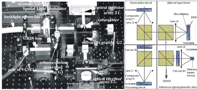
Fig. 1 Practical implementation and functional scheme of the morphological processor.
