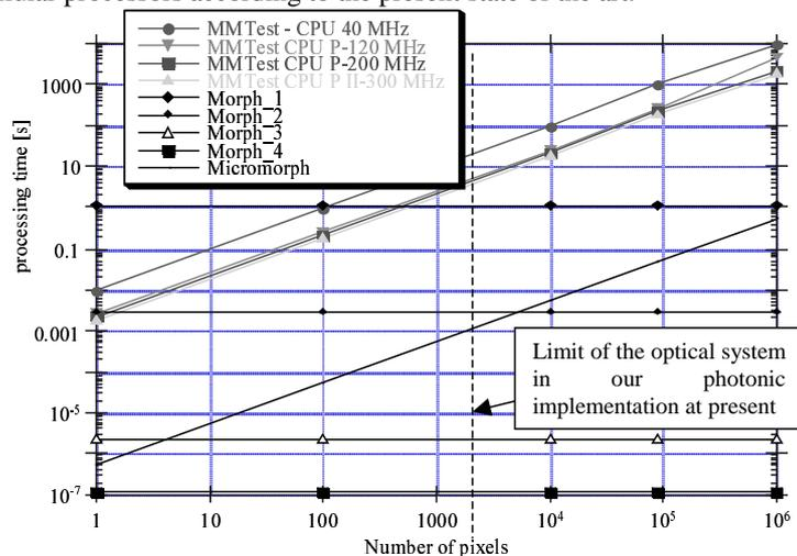
Figure 2 Processing times of dilation and erosion performed with 15x15 structuring element as a function of a number of pixels in an image.
