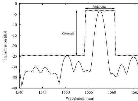
Figure 2: *Definition of crosstalk and ‘peak area’.* The crosstalk is determined by the highest value outside the peak area.
