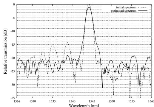
Figure 7: Comparison between initial and optimised transmission responses.
