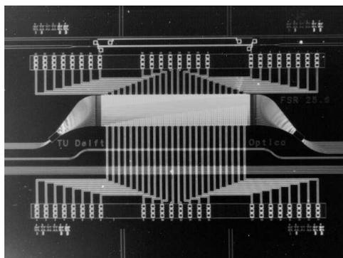
Figure 1: *Photograph of the tunable PHASAR, showing the curved waveguide array, the 48 phase-shifting sections and the electrode patterns.*
