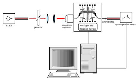
Figure 6: Organisation of the experimental set-up.
