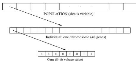
Figure 3: Each gene holds an 8-bit value that is the voltage on one phase-shifting section. Each individual has one chromosome containing 48 genes. A population contains several individuals.
