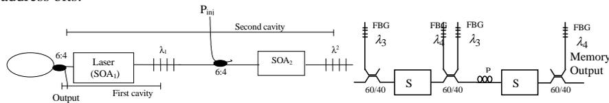
Figure 2: All-optical header processor
