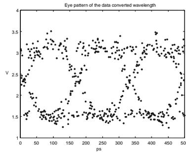
Figure 8: Eye pattern of the converted packet.
