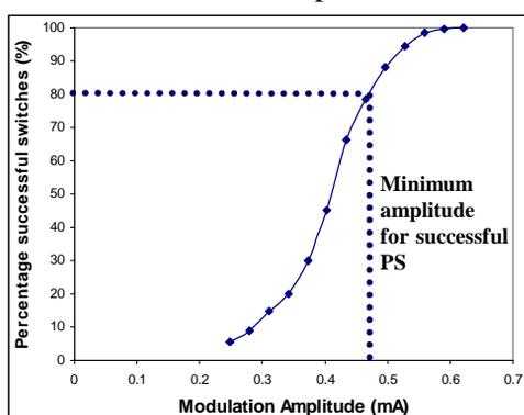
Fig. 1. Fraction of ‘successful’ cycles as a function of the modulation amplitude. The VCSEL is biased at a PS current of 9.85mA and modulated with a 200 kHz sinusoidal signal.
