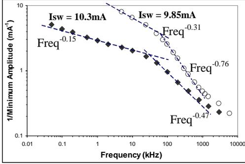
Fig. 2. PS frequency response for switching currents  $I_{sw} = 9.85$  and  $10.3$  mA.
