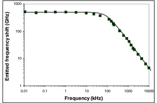
Fig. 3. Thermal frequency response measured at a bias current of  $11.1$  mA and modulation amplitude of  $0.1$  mA (filled squares) and fit to a first-order response function with a cut-off frequency of  $90$  kHz (solid line).
