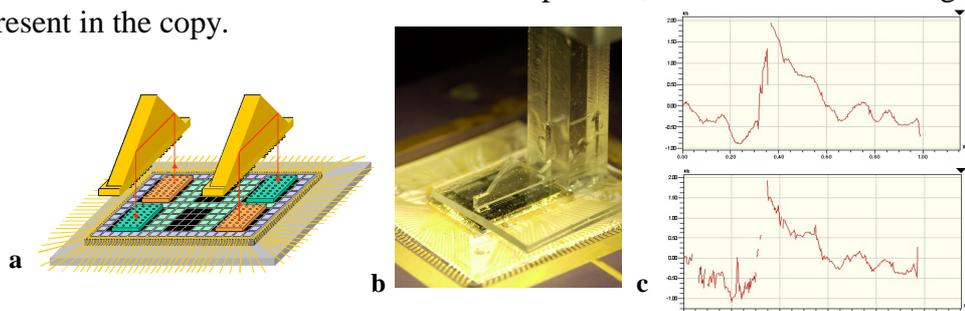
**Figure 3 a. Drawing of optical bridge above the oic chip, b. Image of optical bridge mounted with holder above oic chip, c. Optical surface measurement (roughness of  $3\ \mu\text{m}$  over  $1\ \text{mm}$  length) of a bad mirror of original (lower) and copy (upper).**
