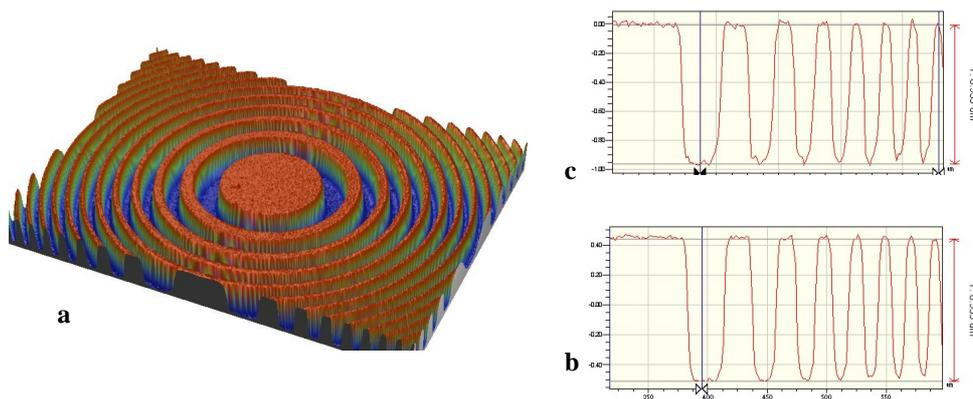
Figure 5 a. Binary Fresnel lens, b. Original lens profile, c. Copy lens profile
