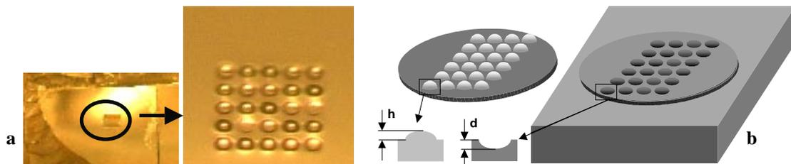
**Figure 2 : a. Picture of the rubber mold with a 5x5 micro lens array, b. Master of the micro lens array and the fabricated rubber mold**
