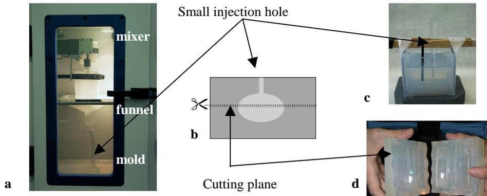
**Figure 1a. Vacuum casting machine, b. Drawing of silicone mold, c. Embedding of the master component in silicone rubber, d. opening of the mold to remove the replicated part in polyurethane**
