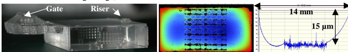
**Figure 4 a. Copy of module with lenses on front and back, b. Measurement on surface of relay module, c. Horizontal surface profile of relay module.**
