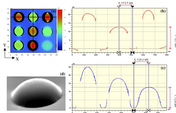
**Figure 3: (a) 3x3 microlensarray with variable sag, constant diameter ( $2a=200\ \mu\text{m}$ ) and pitch ( $P=250\ \mu\text{m}$ ) measured with a non-contact optical profiler (WYKO NT2000); (b-c) X- and Y-2D-plot of the microlensarray respectively; (d) SEM picture of one of the microlenses**
