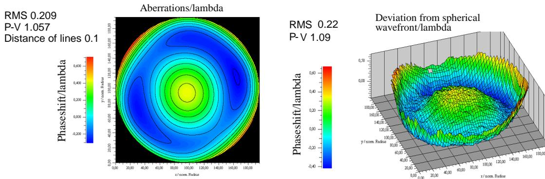
**Figure 4: (a) Aberration/lambda for a 200  $\mu\text{m}$  lens with a height of 23  $\mu\text{m}$ ; (b) Deviation from a spherical wavefront (lambda) for the same microlens**
