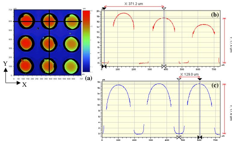
**Figure 2: (a) 3x3 array with columns of uniform 200µm microlenses measured with a non-contact optical profiler (WYKO NT2000); (b-c) X- and Y 2D-plot of the microlensarray respectively**
