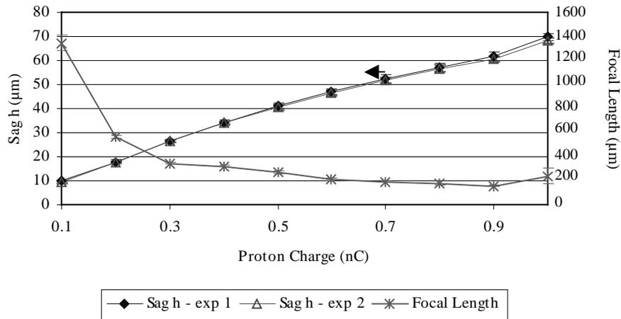
**Figure 1: Sag ( $\mu\text{m}$ ) and Focal Length ( $\mu\text{m}$ ) as a function of the Proton Charge (nC)**
