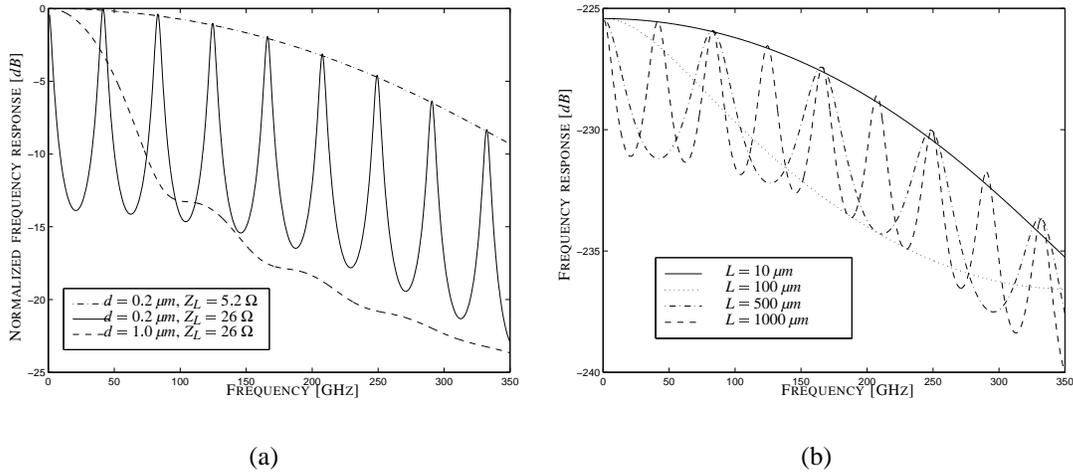
Figure 2: Output voltage of input open-ended TWPD, for (a) three different combinations of intrinsic thickness  $d$  and output load  $Z_L$  and (b) for four different device lengths. (photodetector width  $w = 4 \mu\text{m}$ , optical wavelength  $\lambda = 1.33 \mu\text{m}$ , refractive index  $n = 3.5$ , reverse bias voltage  $V_0 = 10 \text{ V}$ ).
