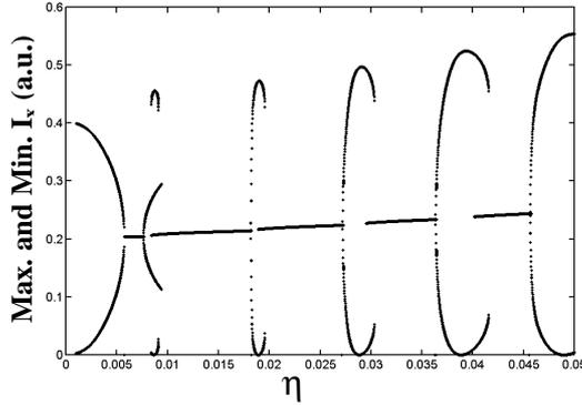
**Fig. 2.** Bifurcation diagram for  $I_x$  as a function of the feedback rate  $\eta$ , for the parameters quoted in the text.
