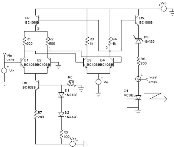
Figure 1 : VCSEL driver circuit scheme consisting of a current source and a differential amplifier stage.
