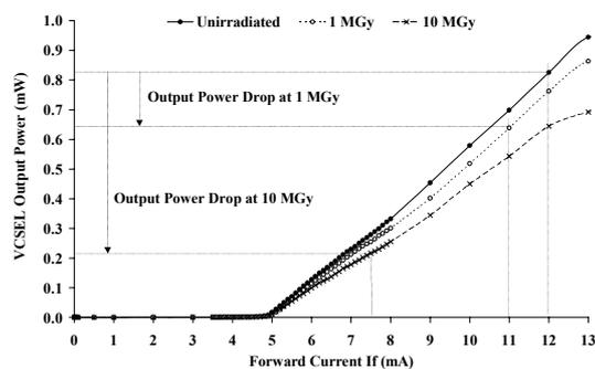
Figure 5 : P-I characteristics of a VCSEL assembly at 0 Gy, 1 MGy and 10 MGy (60 °C). The arrows show the total optical output power decrease due to the radiation effects on both the driver current and the VCSEL.
