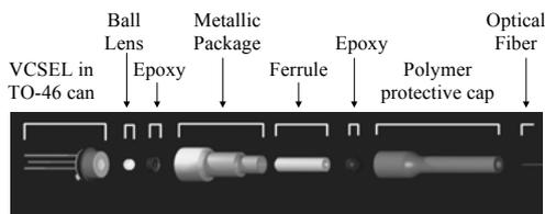
Figure 4 : Exploded view of a pigtailed VCSEL under test, showing the different parts of the assembly.
