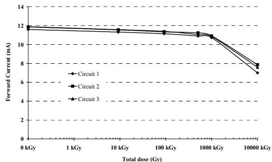
Figure 3 : Forward current measured at 1 MHz on three identical VCSEL driver circuits as a function of total dose at specific total dose values.
