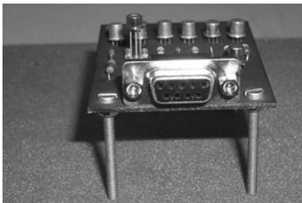
Figure 2 : Driver circuit on polyimide backed PCB
