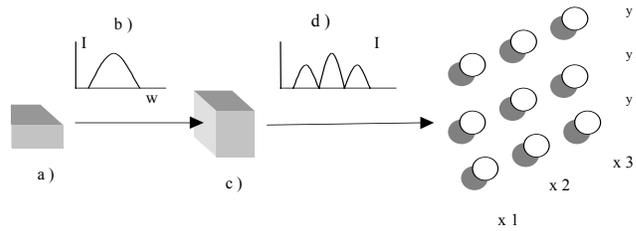
**Fig. 1:** A spectrally sliced broadband light source used to project a 2D spatial pattern with spectral coding. a) Broadband source; b) original spectrum; c) spectral coding; d) sampled spectrum. The 2D pattern on POF entrance with spectral (wavelength) coding.
