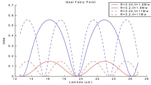
**Fig. 3:** Nonlinear Fabry Perot resonator as an example of the possibilities of coding the information spectrally.
