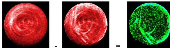
**Fig. 2.** Photographs of two POF output intensity patterns after being processed to reduce noise. The left one was generated by a beam launched near to the center of the core, whereas the second was generated by light injected near to the edge of the core. The image on the right shows the difference between the levels of intensity on each spatial point in these two patterns on its left.
