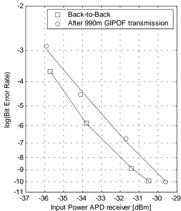
**Figure 2:** Bit Error Rate measurement results 840 nm experiment.
