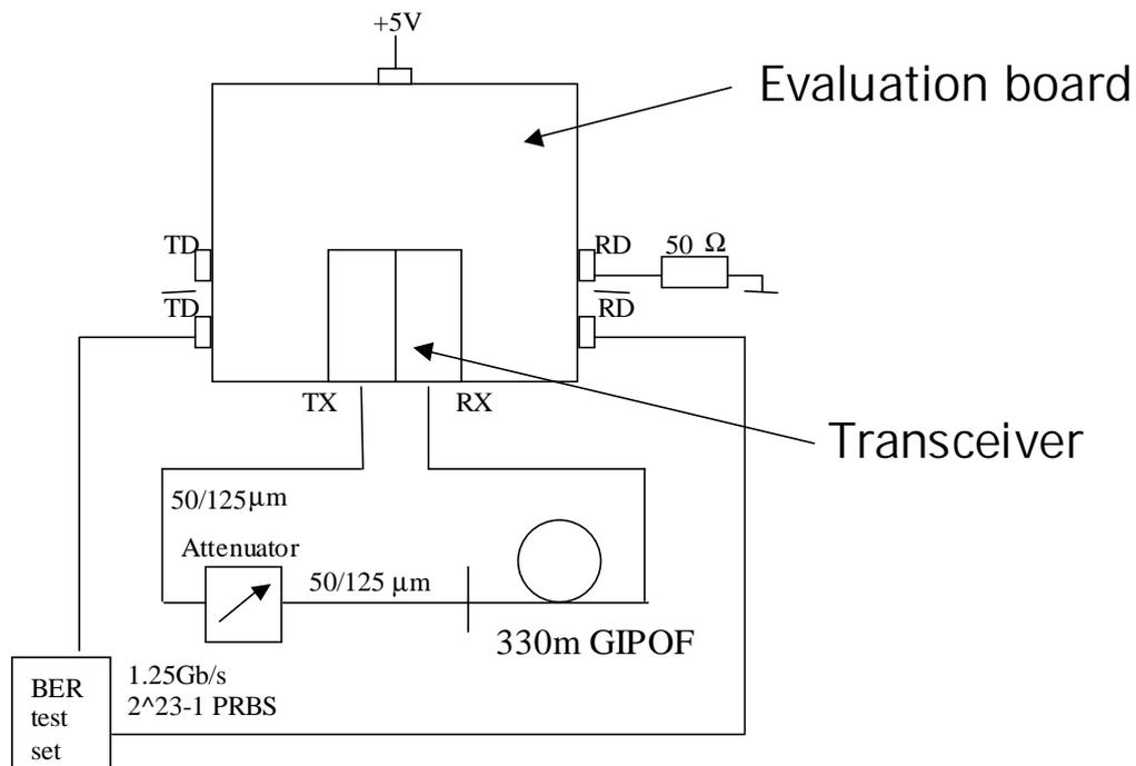
**Figure 3:** Set up of the transmission experiment using a commercially available Gigabit Ethernet transceiver.
