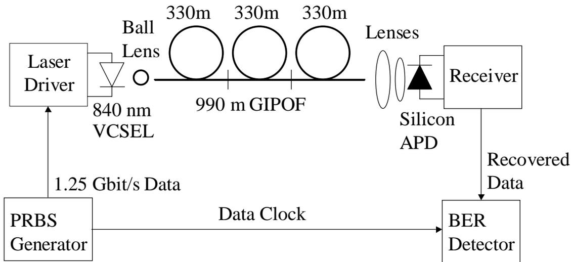
**Figure 1:** Set up of the Gigabit Ethernet transmission experiment at 840 nm.
