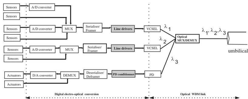
Figure 2: Digital opto-electronic serial link for the ITER instrumentation link
