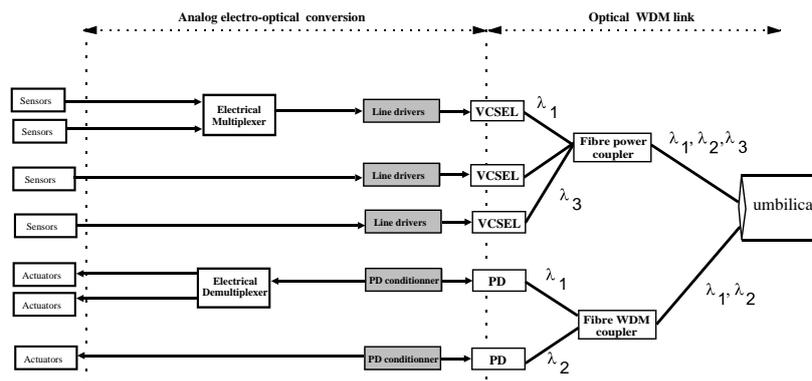
Figure 3: Analog optical parallel link proposed for the ITER instrumentation link
