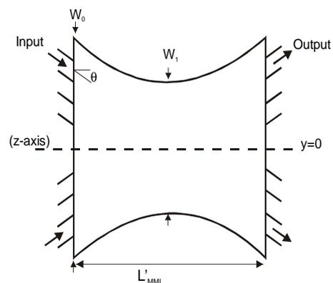
Figure 1: A schematic layout of  $N \times N$  tapered coupler.
