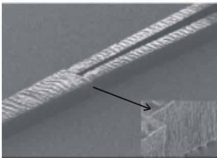
Figure 2: SEM electron micrograph of a  $1 \times 2$  tapered coupler. A close up showing the side-wall roughness is shown in the inset.
