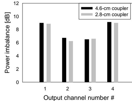
Figure 4: Normalized output power (with respect to the input) of the four channels of two 4 x 4 star couplers with coupler lengths of 46 and 28 mm.
