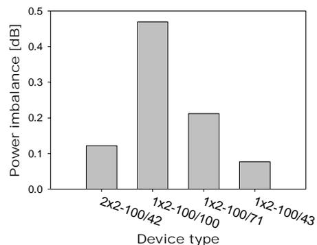
Figure 3: Measured values of the imbalance of different couplers. As a parameter the device type and the start and minimum widths of the tapers are shown.
