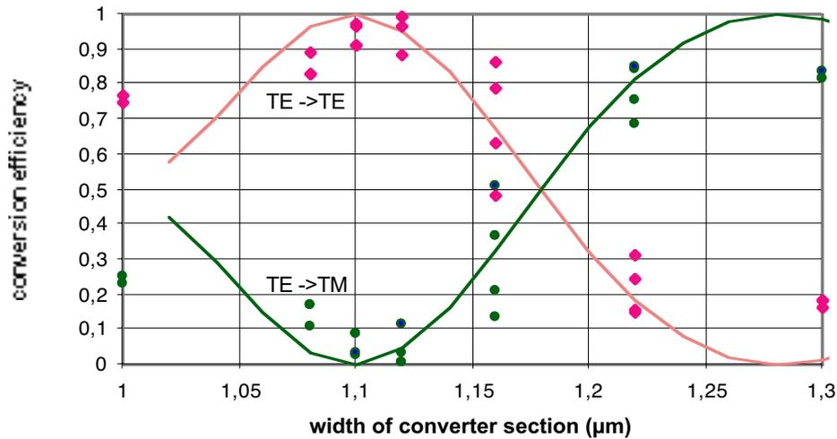
**Fig 4.** Measured TE-TM conversion efficiency and remaining TE polarisation of a single-section polarisation converter. The result of the simulation (continuous curves) are shown for comparison.
