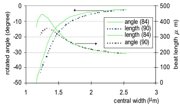
**Fig. 2** The polarisation angle of the TE quasi mode and the interaction length as function of the center width of the converter section. Dotted:  $84^\circ$  angle; solid:  $90^\circ$  angle (vertical) of the side-wall.
