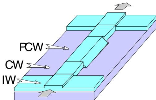
**Fig 1.** Schematic structure of the single-section polarisation converter.
