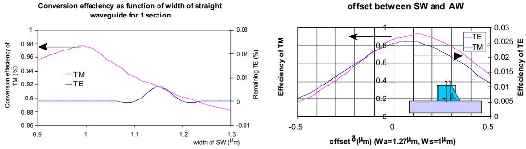
**Fig 3.** Calculated coupling efficiency from the deep-etched waveguide to the converter section as function of the width of the deep-etched waveguide(left) and of the offset of this waveguide with the converter section(right).
