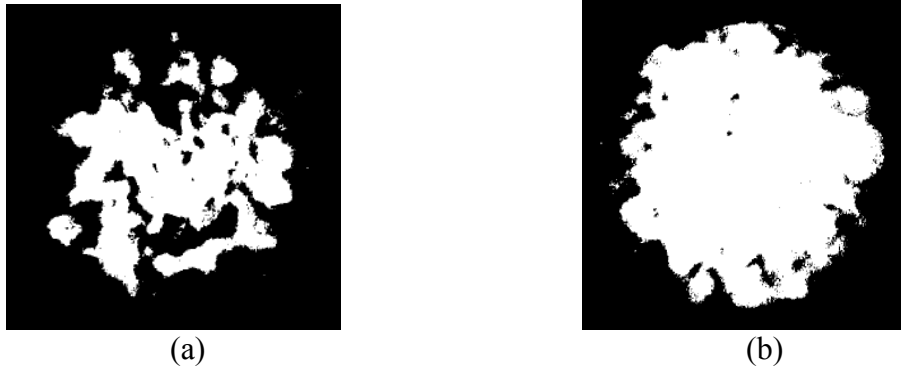
Fig.2 Photographs at the output of the optical fibre. (a) a single beam (b) two interaction beams
