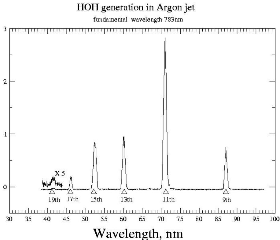
Fig. 3: Results of high-order harmonic generation in a pulsed jet of Argon gas at a fundamental wavelength of 783 nm. The input energy is 225 mJ in 320 ps pulses. Extreme ultraviolet radiation down to 42 nm is produced. Note that the width of the resonances is determined by the grating-slit setup and that it does not reflect the bandwidth of the XUV-radiation.
