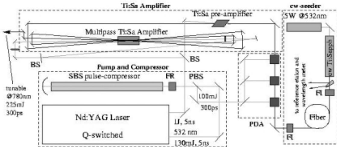
Fig. 2: Layout of the entire laser system, delivering at the output pulses of 225 mJ/pulse, with 320 ps duration, a 1.5 GHz bandwidth, an  $M^2$  beam profile value of 2.5, and at a 10 Hz repetition rate. The subsystems are schematically drawn in boxes; the seed laser determining the frequency at the right, the pulsed dye-amplifier (PDA) section, the pump laser and the SBS-compression cell at the bottom, and the Ti:Sa amplifying stages at the top.
