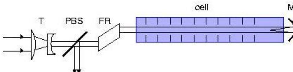
Fig. 1; SBS-compressor setup consisting of a cell of 1 m length filled with clean water, and some optics. The two lenses forming the telescope (T) bring the beam to the optimum power density, the Faraday rotator (FR) circularly polarizes the laser beam, and the mirror (M) retroreflects the beam into a focal zone where the SBS-process starts, resulting in a phase-conjugate back-reflected beam, which is separated by the polarizing beam splitter (PBS) from the incident beam.
