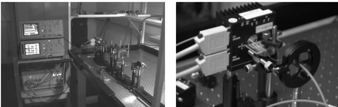
Fig. 2.: (left) Proof-of-principle demonstrator of the free-space laserlink. (right) Coupling of the laserbeam into the fiber using a grin lens, components are aligned using a custom fabricated PMMA Vgroove.
