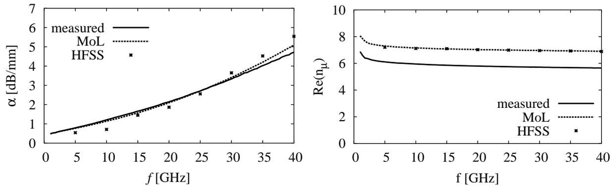
Figure 3: Measurements (solid line), MoL-simulations (dashed line) and HFSS-simulations (crosses) of the microwave attenuation  $\alpha$  (left) and of the microwave index  $n_\mu$  (right) for a phase-shifter with a signal line width  $w_{sig}$  of  $6 \mu\text{m}$ .
