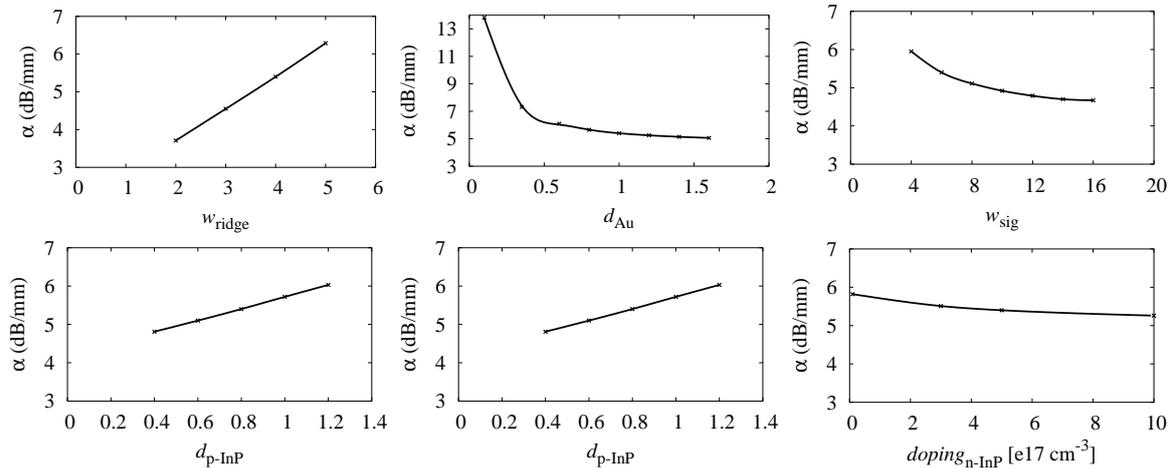
Figure 2: RF-attenuation at 40 GHz as a function of ridge width (top left), gold thickness (top middle), signal line width (top right), p-cladding thickness (bottom left), buffer thickness (bottom middle) and buffer doping (bottom right). Other parameters are as in the optimized design.
