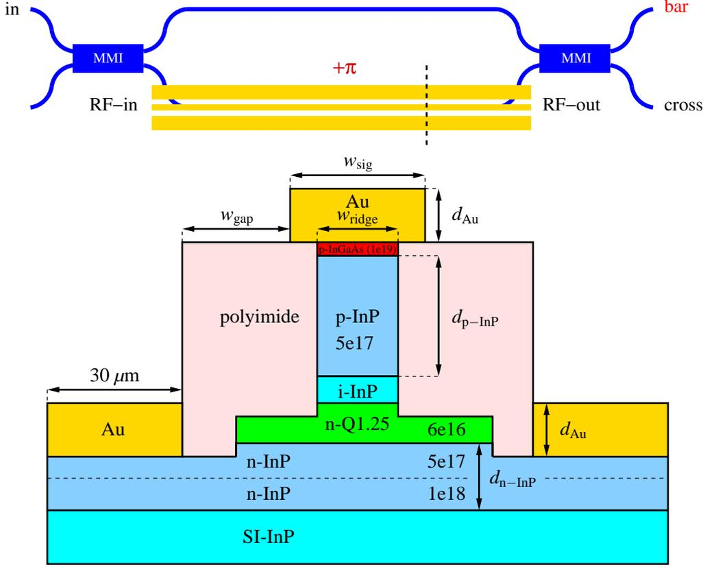
Figure 1: Top view and cross-section (at dashed line) of a travelling-wave electro-optic modulator.
