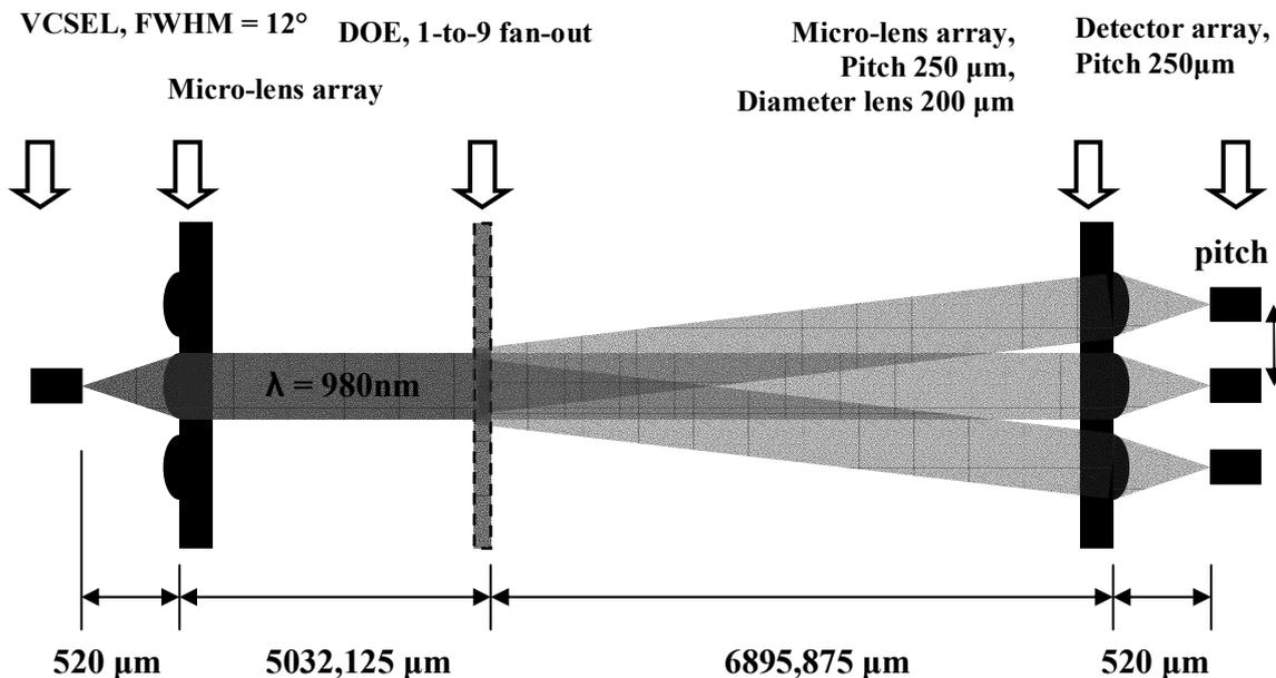
Fig. 1: Virtual Lab simulation model of the optical pathway block equipped with DOEs. The model includes a VCSEL, a 3 by 3 lenslet array, a DOE for 3 by 3 spot fan-out functionality, a second focusing 3 by 3 lenslet array, and a detector plane.
