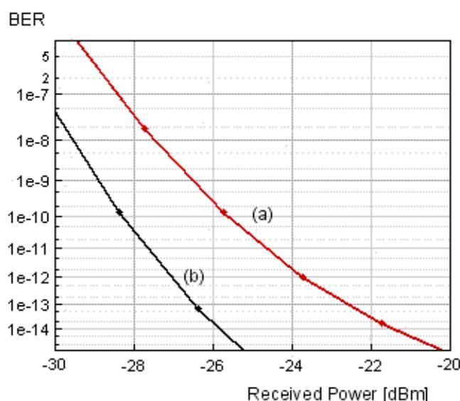
Figure 5: 8 APs on a ring: (a) With normal 2x1 switches, (b) With dilated switches
