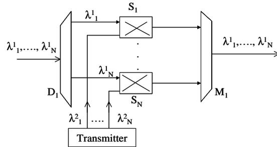
Figure 3: Model for analyzing Inband Crosstalk
