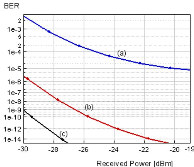
Figure 4: Scalability: (a) 10 APs, (b) 8 APs, (c) 6 APs, on a single ring
