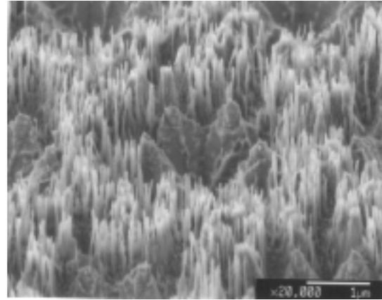
Fig. 4. SEM image of GaN epitaxial layer after PEC etching.
