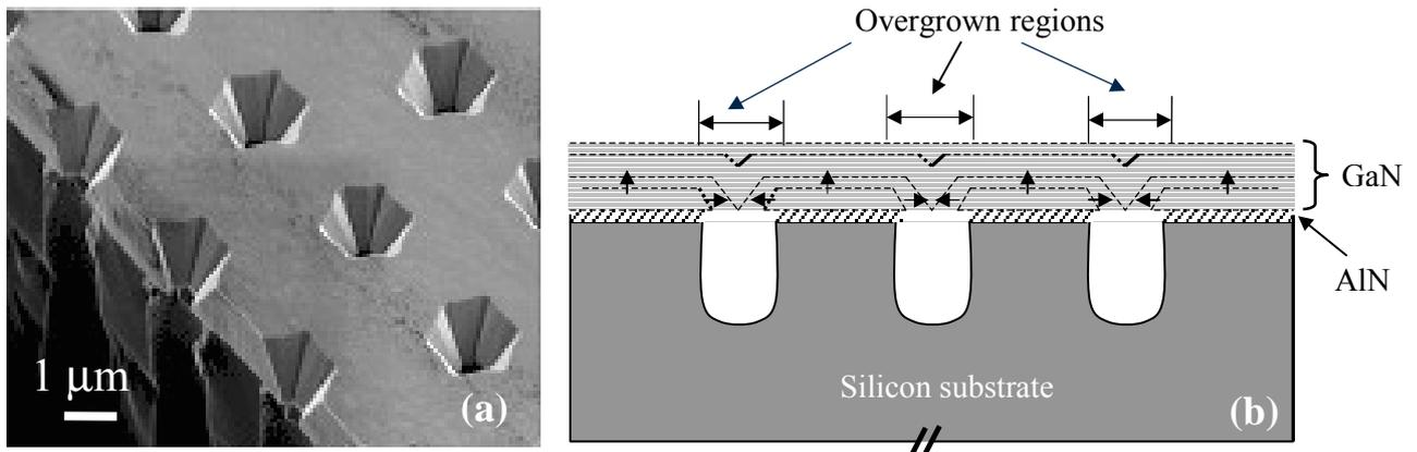
Fig. 2. (a) SEM image of 2μm-thick GaN layer and schematisation of the two-dimensional evolution of the deposition (b).
