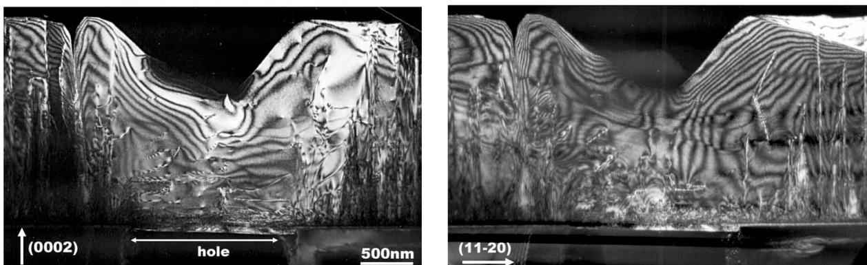
Fig. 3. (0002) and (11-20) dark field cross-section TEM images of GaN laterally grown over the opening in the silicon substrate.
