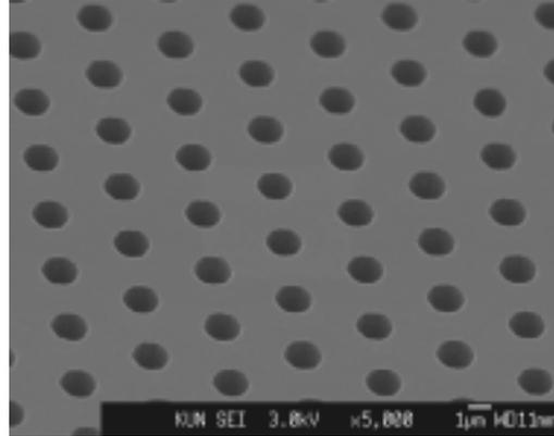
Fig. 1. Top view Scanning electron microscope (SEM) image of the structured Si (111) substrate.
