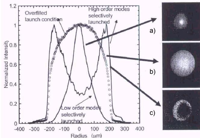
**Fig. 3 Near-Field Patterns at output of multimode POF, depending on launching conditions [4]**
