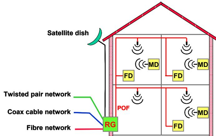
**Fig. 4 Transparent In-House Network with Polymer Optical Fibre, integrating wireline and wireless services in a single infrastructure**
