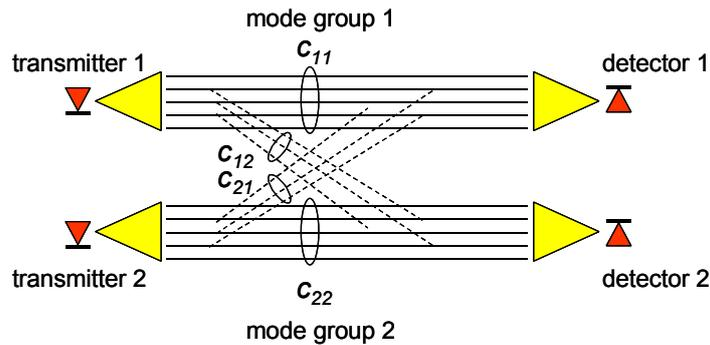
**Fig. 2 Modelling the optical system transfer function (for  $N=M=2$ )**
