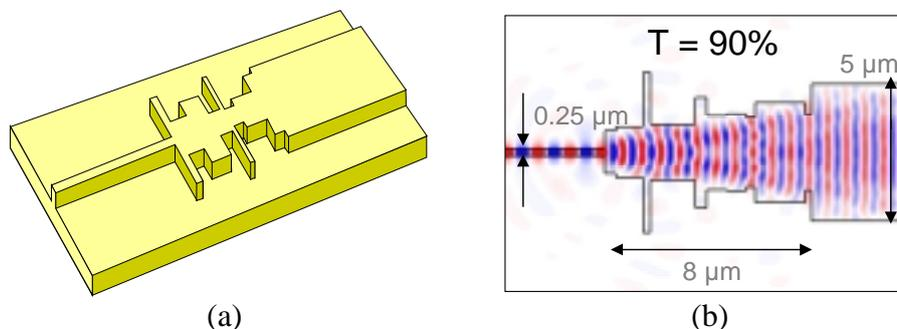
**Fig. 3: (a) schematic 3-D view of interference coupler (b) 2-D field plot of a similar structure (magnetic field perpendicular to surface)**
