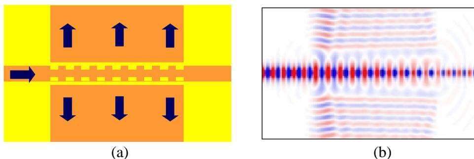
Fig. 1: (a) 2-D simulation plot of the in-plane grating coupler (b) corresponding field plot (magnetic field perpendicular to surface)
