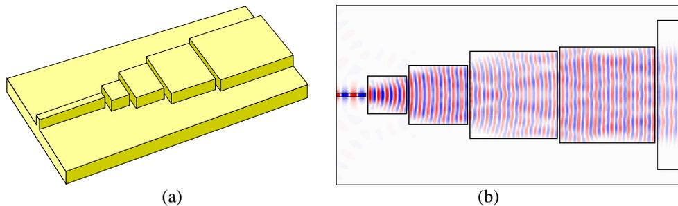
**Fig. 2: (a) schematic 3-D of a resonance coupler (b) 2-D field plot of a similar structure (magnetic field perpendicular to surface)**
