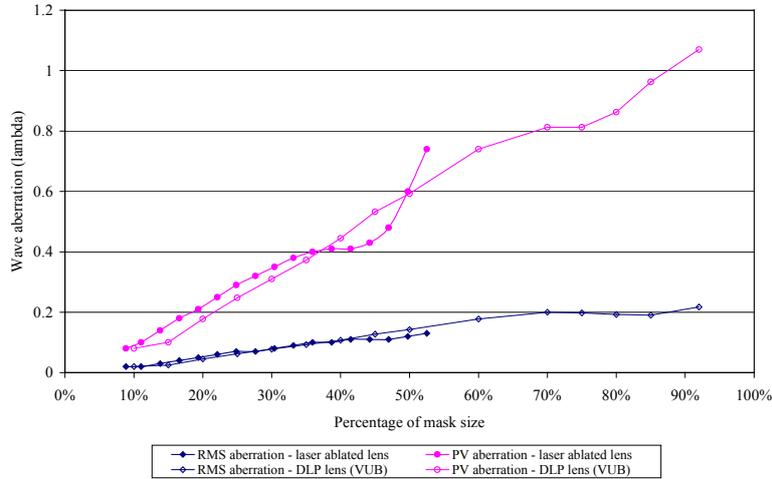
**Figure 2: The influence of the mask size on the RMS and PV wave aberrations ( $\lambda$ ) for a laser ablated microlens and a DLP lens (VUB) with the same characteristics ( $D= 200 \mu\text{m}$ ;  $f= 1283 \mu\text{m}$ )**
