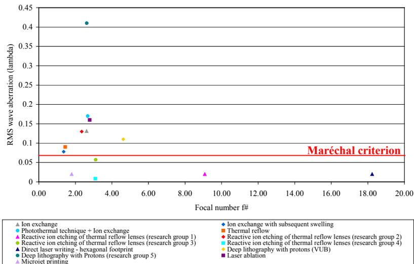
**Figure 3: RMS wave aberrations ( $\lambda$ ) as a function of the focal number  $f\#$  for the highest-quality microlens of each fabrication technique**
