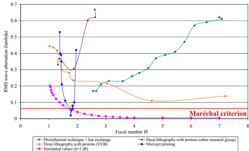
**Figure 1: RMS wave aberrations ( $\lambda$ ) as a function of the focal number  $f\#$  for all characterized microlenses**
